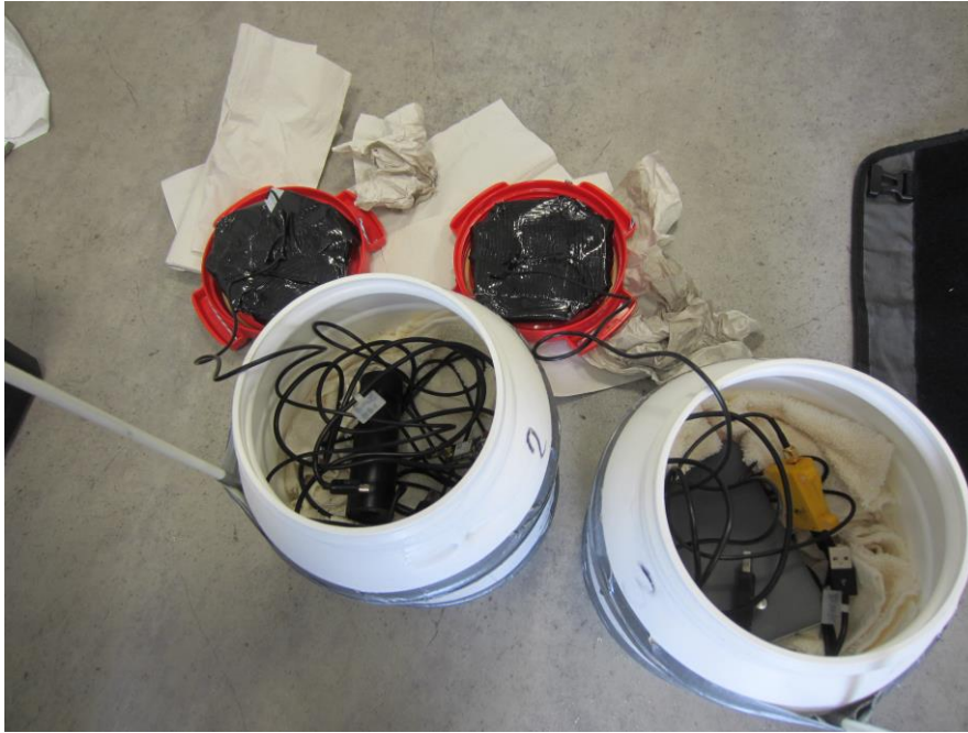
Figure 1: Two buoys equipped with single-frequency GNSS hardware.
