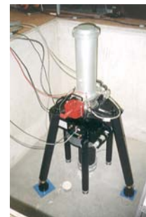
FG-5 absolute gravimeter in the gravimetric bunker at Westerbork
