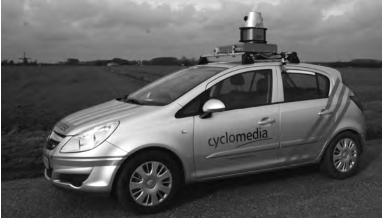
Figure 4. The CycloMedia ground-based image acquisition platform DCR7.
