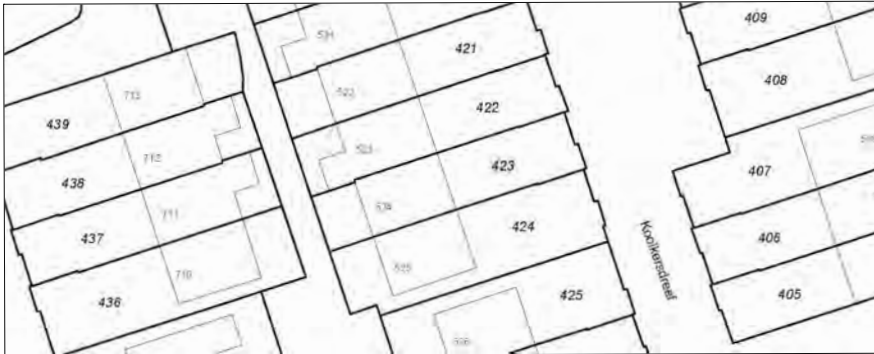
Figure 1. Excerpt from a modern parcel based cadastral map (boundaries fat line; buildings thin line).
