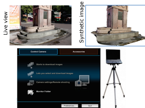
Fig. 5.6: Software-hardware illustration of the guiding system.
