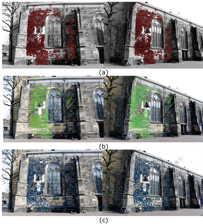
Fig. 7.12: (a) Image correspondences using our guided matching. (b) Image correspondences using VSFM software. (c) Image correspondences using Agisoft photostan software.
