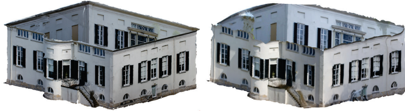
Fig.1.2: Automated 3D model from (37) still images (left) and 3D model from (178) video frames (right).
