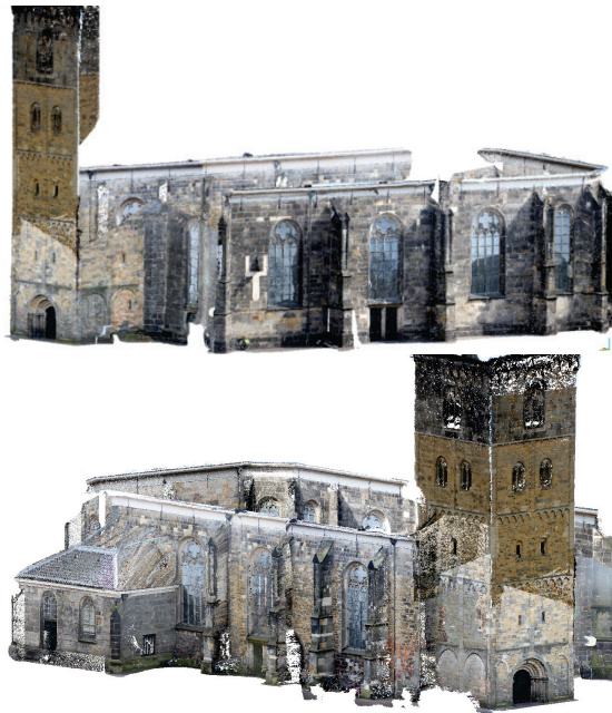
Fig.7.14: The dense textured point cloud of the church using MICMAC.
