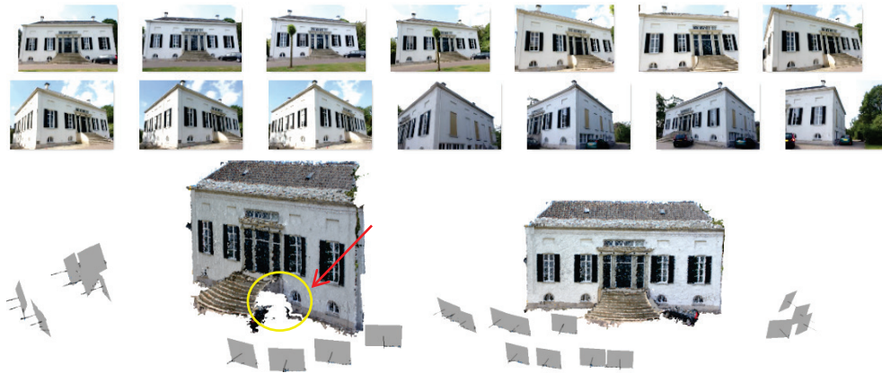
Fig.6.13: Façade dense point cloud.
