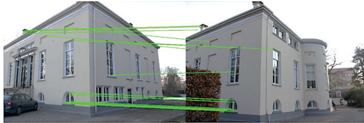
Fig.1.3: Repetitive texture patterns affecting the tie points matching and leading to wrong correspondences.
