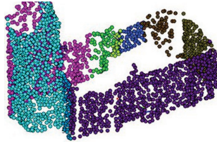
Fig.7.5: The segmentation of the church rough point cloud.
