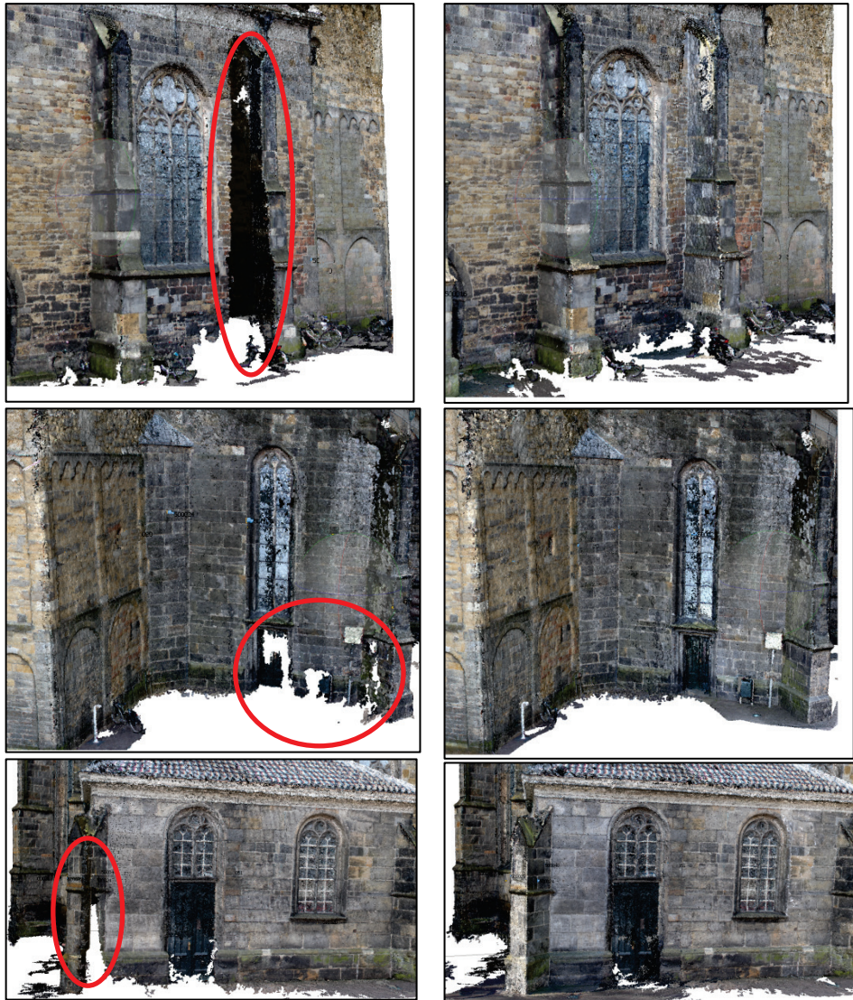
Fig. 7.23: Dense point cloud illustrates the gap in different parts of the church before (left) and after (right) gap detection and point cloud completeness.
