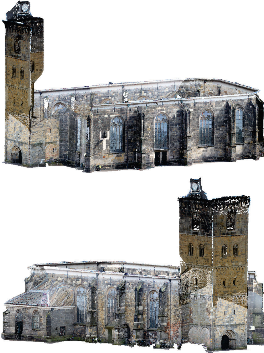
Fig.7.24: The complete point cloud of the church from a layman camera height.
