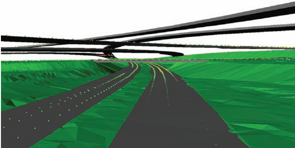
Figure 4-8 Height differences between reconstructed model and reference data, shown as dots at paint strip locations.
