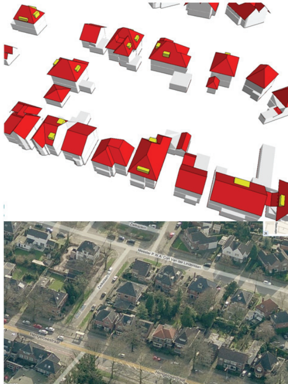
Figure 7-4 Top: Variety of complex 3D building models in Zwik area (Ens 1). Bottom: oblique image [bing.com].
