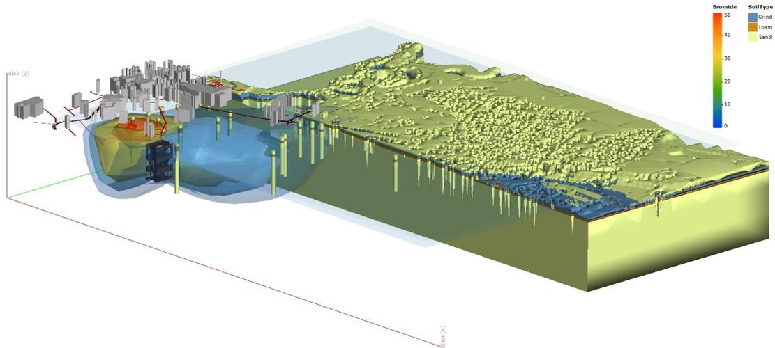
**Figure 5.14:** 3D representation of the subsurface of the case area
