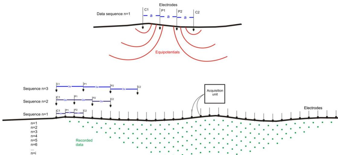
**Figure 2.16:** Typical setup for an ERT survey
