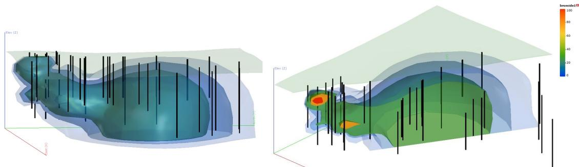
Figure 5.12: Contamination plume of concentrations bromide
