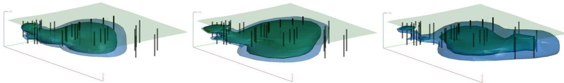
Figure 5.1: 3 snapshots in time of a contamination plume
