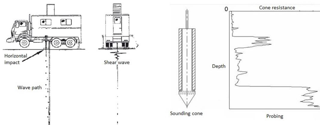
**Figure 2.13:** Probing technique and output
