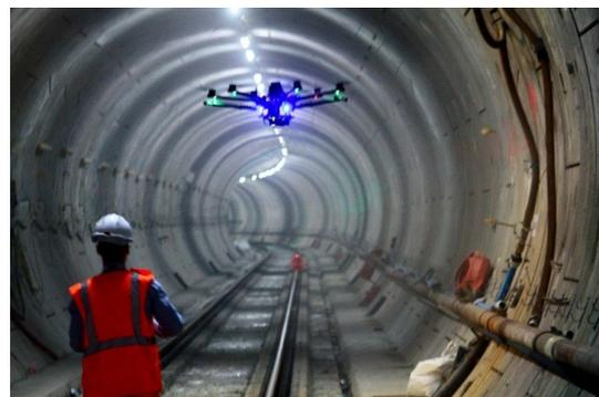
**Figure 2.10:** 3D tunnel scanning
