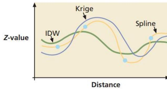
**Figure A.12:** IDW, kriging and spline
