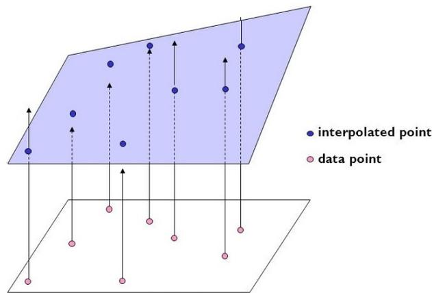
**Figure A.8:** Fitting a trend surface
