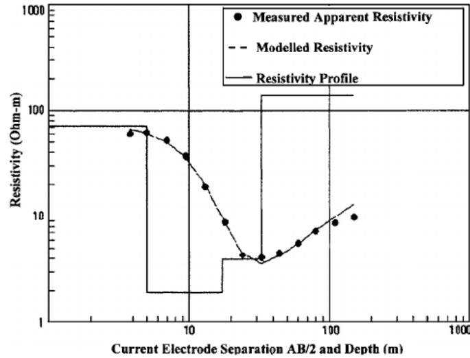
**Figure 2.15:** Typical output of VES measurement
