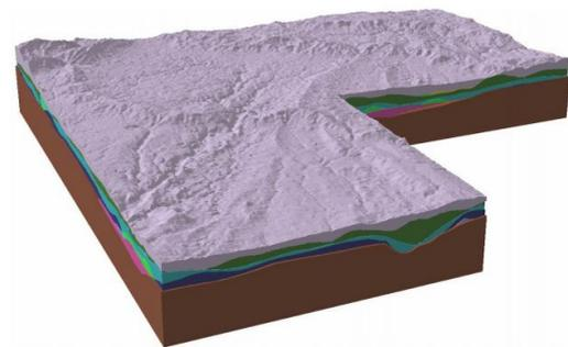
**Figure 4.2:** 3D soil type block diagram
