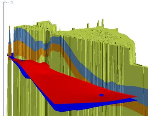
Figure 5.11: Groundwater relative to lithology
