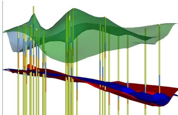
Figure 5.10: Groundwater levels of two time periods
