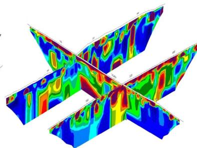
Figure 5.3: ERT profiles as point data
