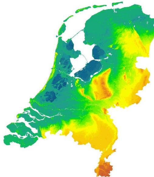
Figure 2.7: Ground level height (AHN)
