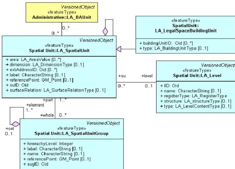
*Figure 65 The spatial unit class and its association to LA\_BAUnit in the proposed CLIS data model, based on the LADM (Elia et al, 2011).*
