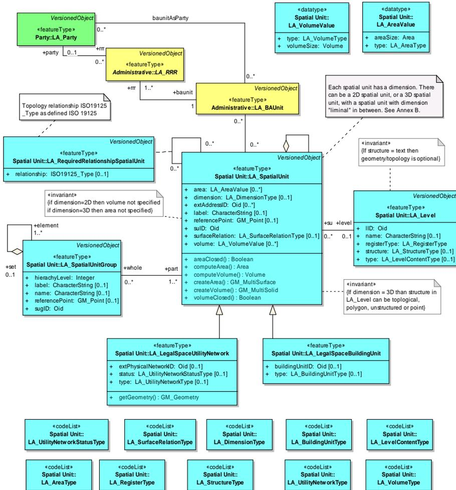
Figure 33 LADM Version C Spatial Unit Package with associations to other core classes (ISO, 2011c).
