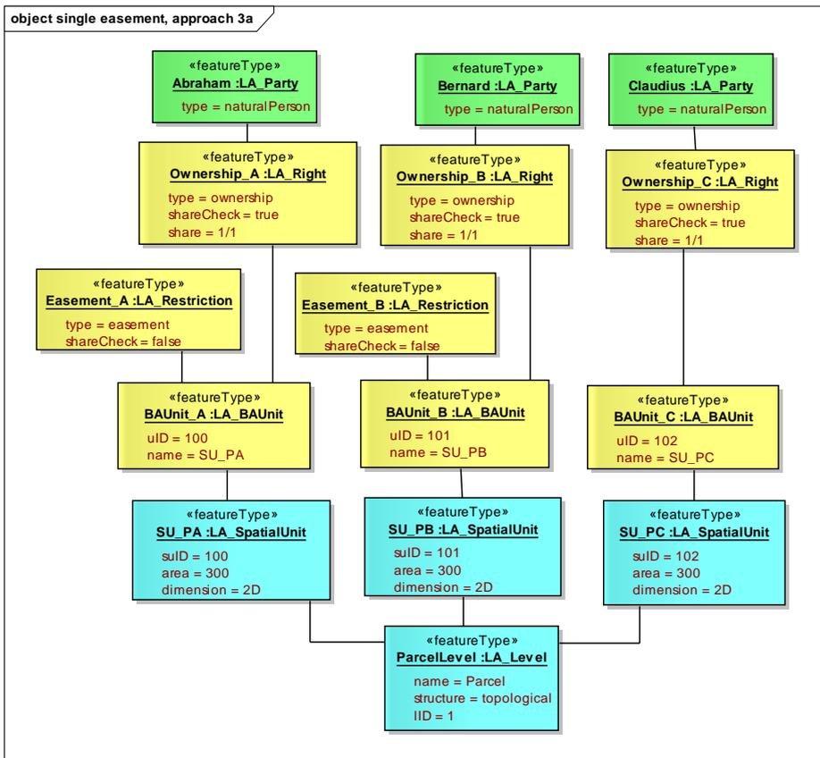
Figure C-1 LADM instance diagram: single easement with no geometry, no party.
