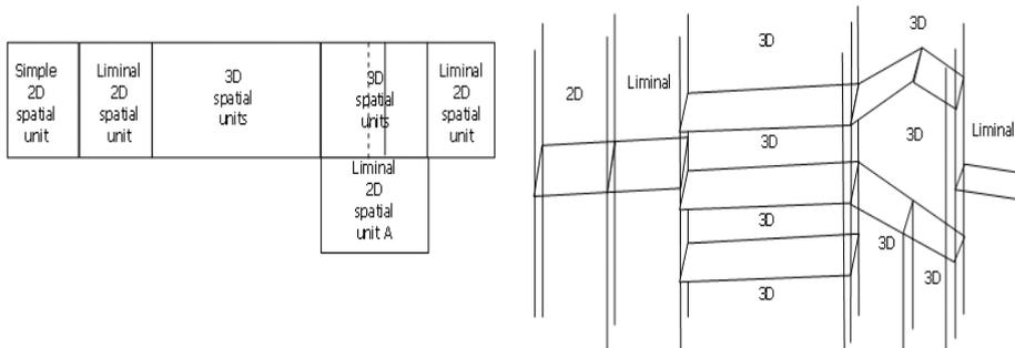
*Figure 37 left: top view of mixed 2D/3D representations, right: side view showing the mixed use of boundary face strings and boundary faces to define both bounded and unbounded 3D volumes (Lemmen et al, 2009a); figure designed and created by Rod Thompson.*
