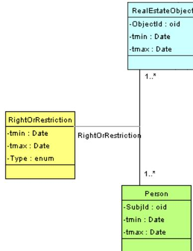
Figure 20 Core of Version A: Person, RightOrRestriction, RealEstateObject (Lemmen et al, 2003c).
