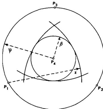
Fig. 3. Definition of domain of common observability between stations  $P_1$ ,  $P_2$ ,  $P_3$  and  $P_4$ .
