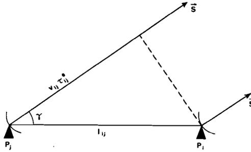
Fig. 1. Basic geometric relationship in VLBI with sources at infinity.
