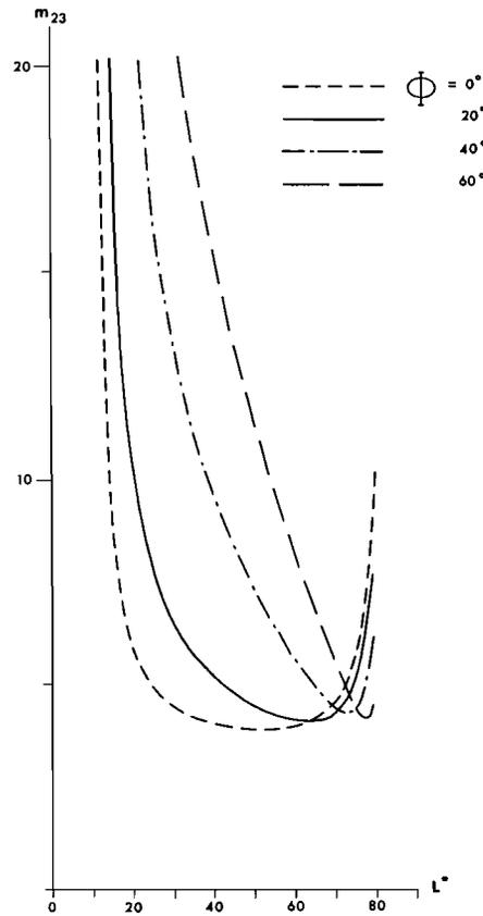
Fig. 6. Reduced standard deviation  $m_{23}$  for some values of azimuth  $\Phi$ .  $\delta^I = 35^\circ$ ;  $\delta^{II} = 55^\circ$ .  $z = 75^\circ$ .  $\psi = 30^\circ$ .
