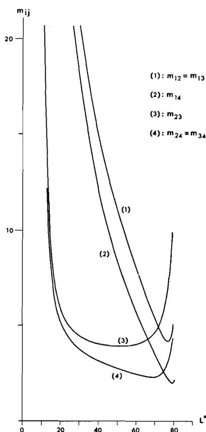
Fig. 4. Reduced standard deviations of interstation distances in model station configuration with  $\delta^I = 35^\circ$ ;  $\delta^{II} = 55^\circ$ .  $z = 75^\circ$ .  $\psi = 30^\circ$ .  $\Phi = 0^\circ$ .
