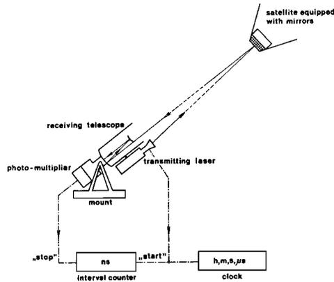
Principle laser distance measurement
