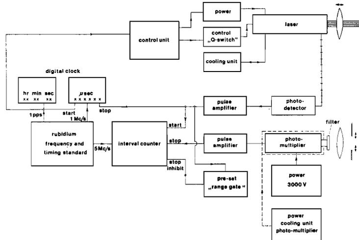
Diagram laser distance measurement equipment
