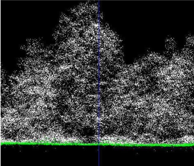
*Figure 5. Classification of terrain (green) in the point cloud of an area with dense vegetation. Because of this vegetation, the AHN requires the acquisition to be in the winter (image Fugro Aerial Mapping).*
