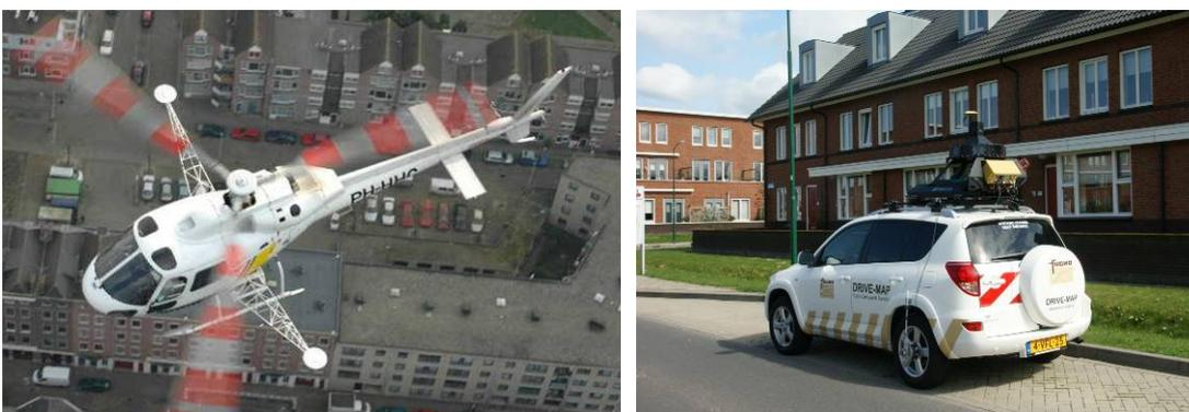
Figure 2. FLI-MAP (helicopter based) and DRIVE-MAP.
