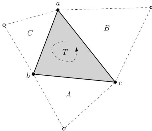
Figure 2. With the triangle-based data structure, the triangle  $T$  has 3 pointers to its 3 vertices  $a$ ,  $b$  and  $c$ ; and to its 3 neighbouring triangles  $A$ ,  $B$  and  $C$ . The pair vertex-triangle is organised in such a way that for instance  $a$  is ‘opposite’ to  $A$ .
