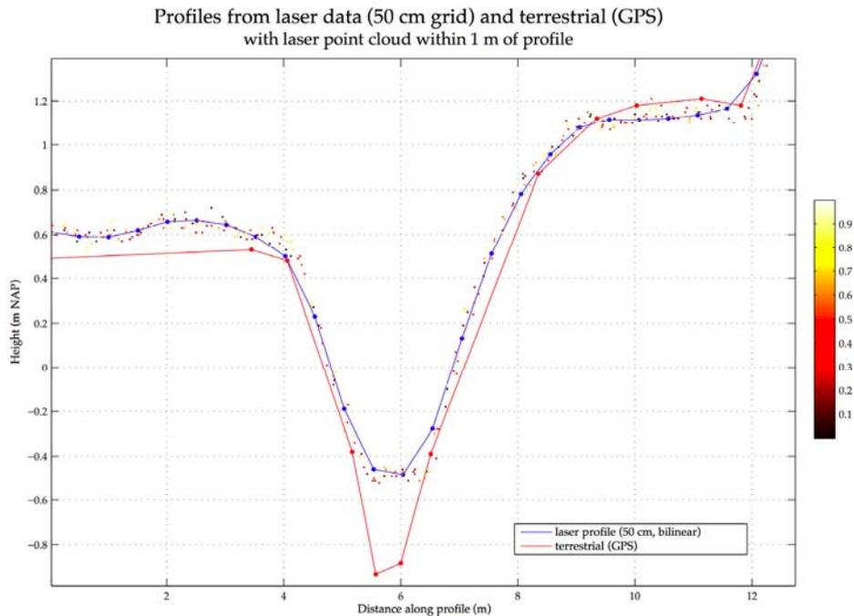
Figure 9. The profile near the ditch at the toe of the dike, plotted as described in Figure 8. The laser data reflect the topography with more detail than the terrestrial profile, although the height makes a significant excursion that cannot be judged without further knowledge. The depth of the ditch can only be measured with a terrestrial technique.
