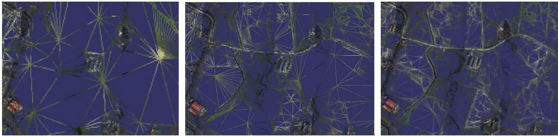
*Figure 2: Screenshots in wireframe mode of the same area in the AHN2 terrain as seen from a large viewing distance (left, scaled) through to a small distance (right). As the viewing distance decreases, a different level-of-detail is visible with more accurate triangulation and higher resolution texture information.*
