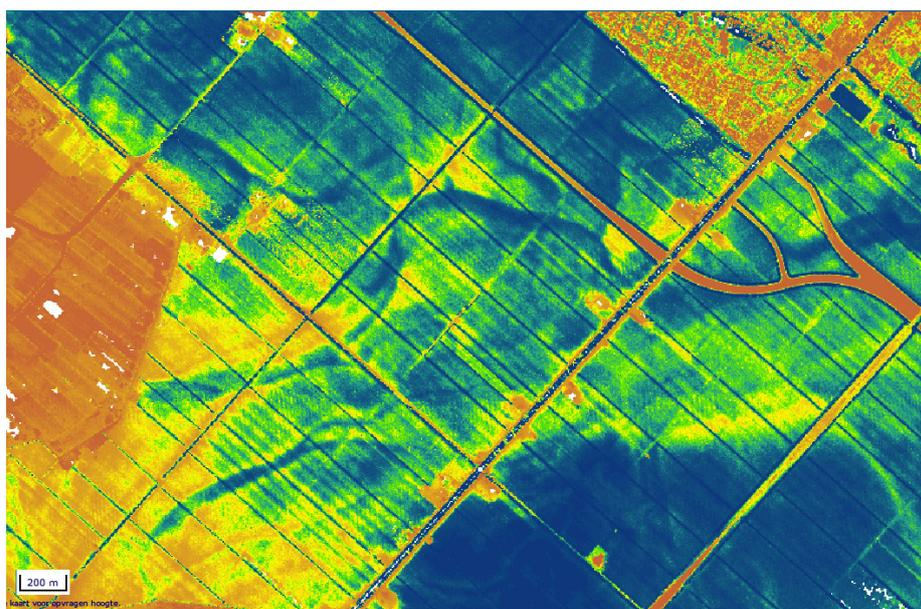
Figure 4. For many applications, the point density and accuracy of the AHN-1 suffices. With the AHN viewer at [ahn.nl](http://ahn.nl), any user can explore height data in sufficient detail to discover unexpected features in the landscape himself. Just by adapting the legend of the viewer at the world wide web, the author ‘discovered’ that the 180 sq km Haarlemmermeer polder he lives in is not as flat as it seems. The 1997 1pt/8m<sup>2</sup> data is sufficient to uncover old streams.
