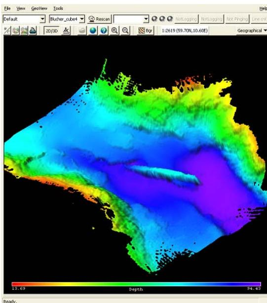
Figure 13. A terrain model made from depth points.
