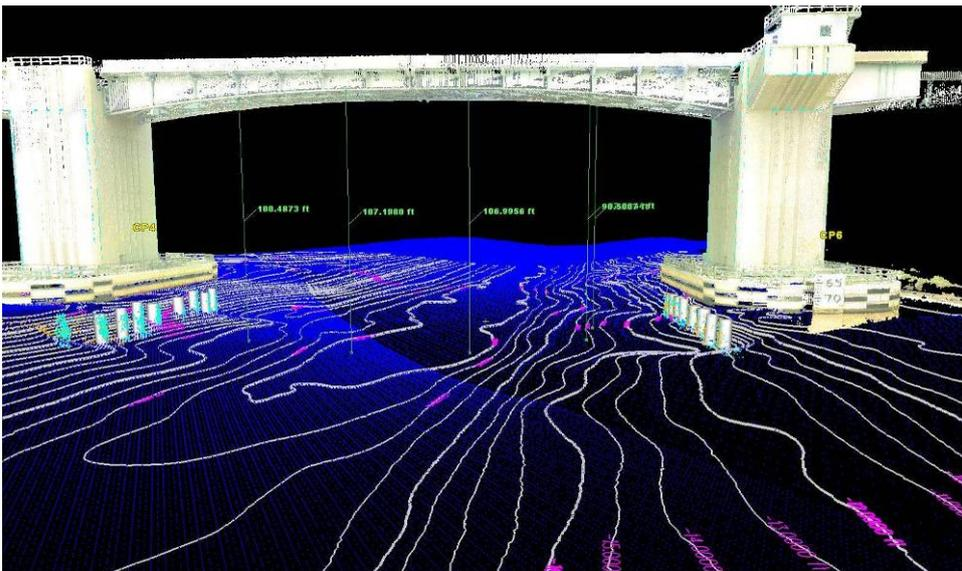
Figure 4. Combination of terrestrial and acoustic data.
