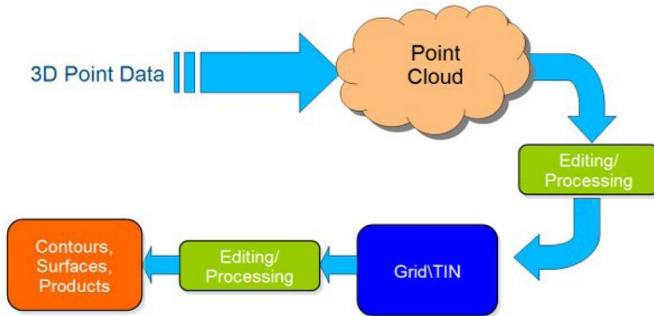
Figure 1. A typical bathymetric point post-processing workflow.
