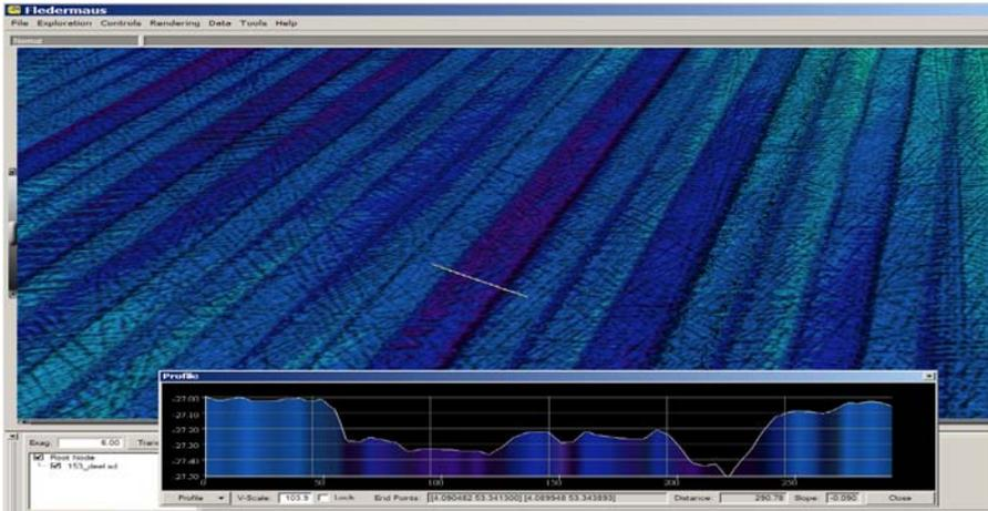
Figure 3. Example of tidal correction error artifacts.
