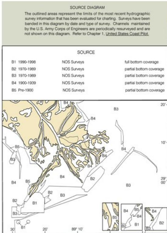
Figure 4. Example source diagram (courtesy NOAA).
