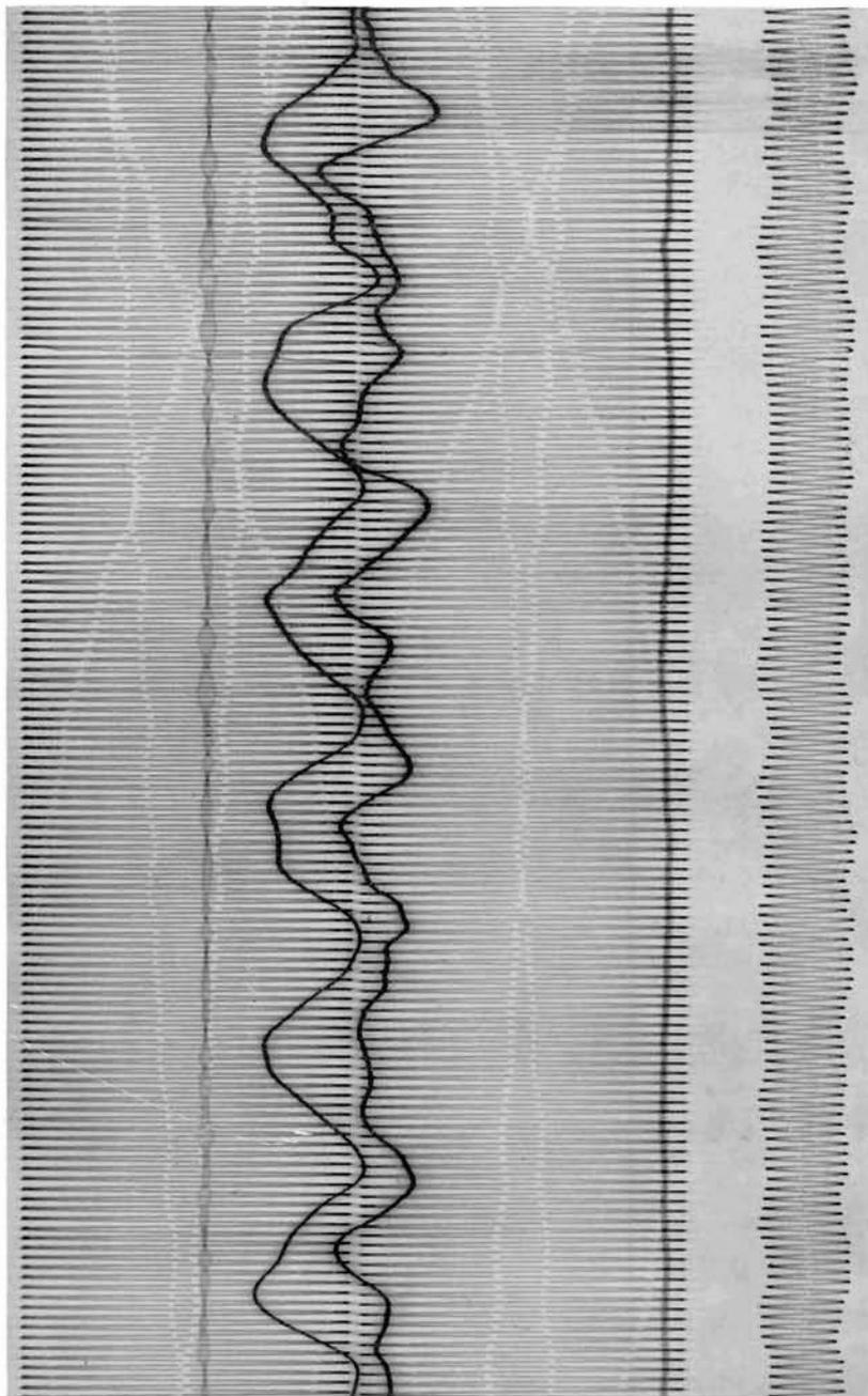
Plate III. No 4 *B*, voyage O 13, depth 37.5 m, course slowly changing from  $190^\circ$  (top) to  $170^\circ$  (bottom); same record as Plate VI but the undamped free swinging of the slow pendulums makes it difficult to measure the wave-period of 14 sec present in the fluctuations of the second-mark curves and clearly visible in Plate VI.
