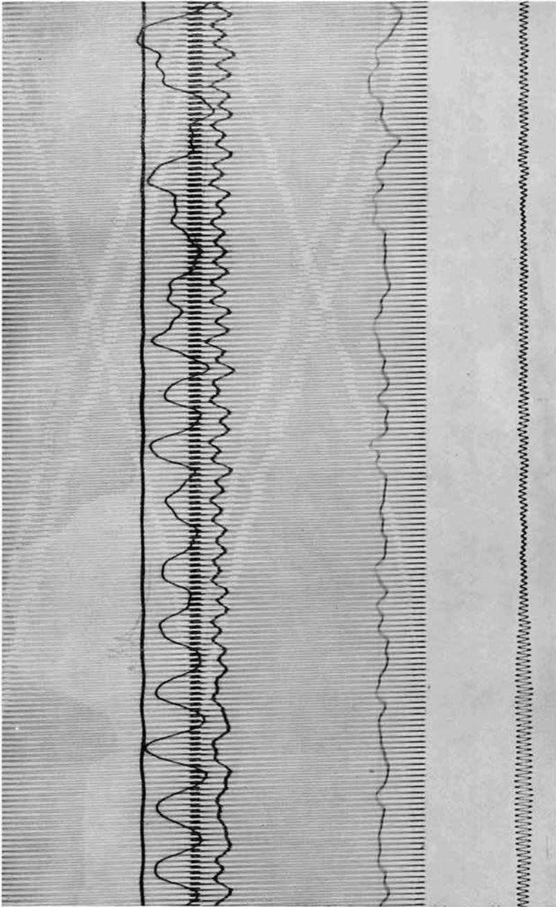
Plate IV. No 1 A, voyage O 19, depth 17.5 m, course  $180^{\circ}$ ; same record as Plate VII. The record shows a strong damping of both slow pendulums, which at the top have amplitudes disappearing quickly towards the bottom. At the bottom the wave-period of 10 sec is clearly visible in the left slow pendulum record.
