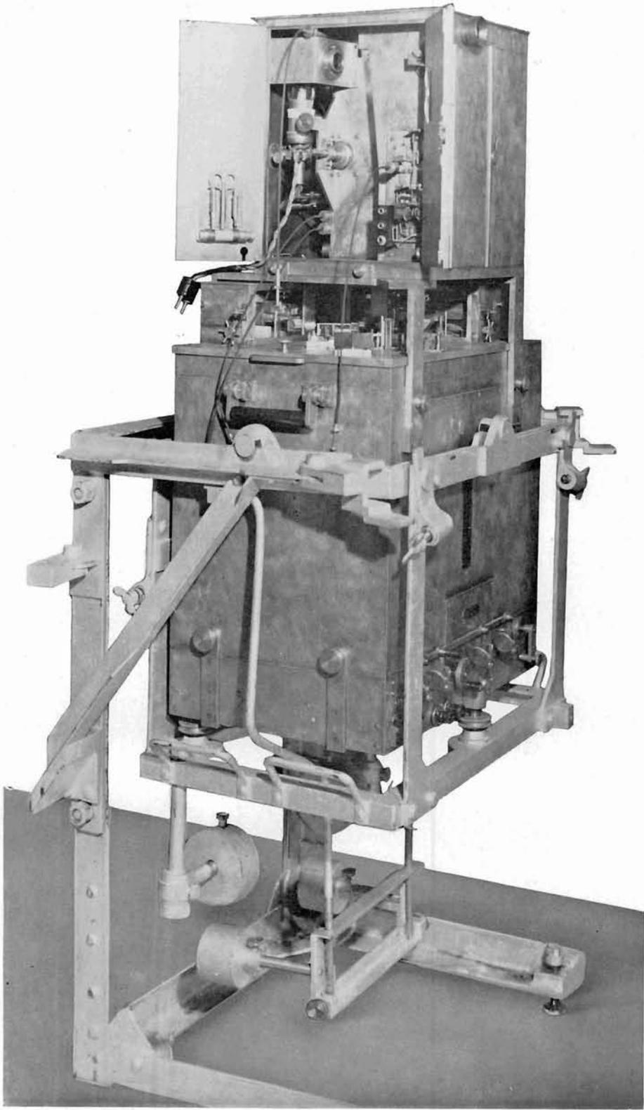
Plate II. Pendulum apparatus for gravity determinations at sea; the slow pendulum apparatus of Plate I is introduced between the recording and the pendulum apparatus. New gimbal system of which the swinging-period for both directions can be independently adjusted.
