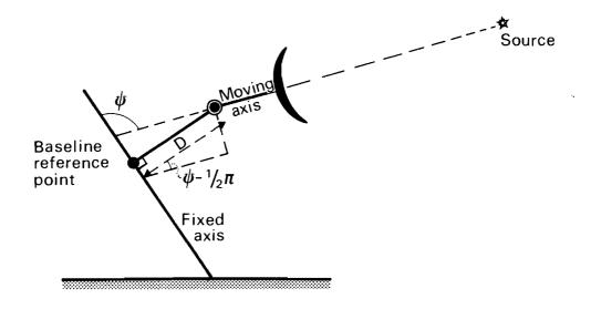
Figure 6: Telescope Axis Offset
