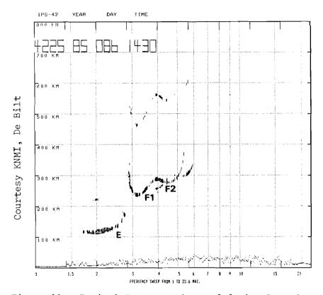
Figure 11: Typical Ionogram observed during Day-time
