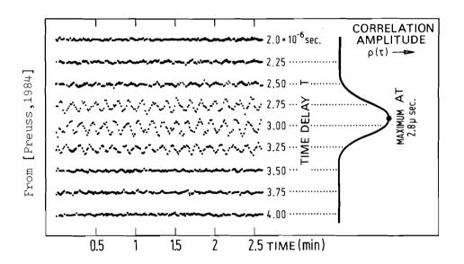
Figure 3: Stopped Fringes and Correlation Amplitude
