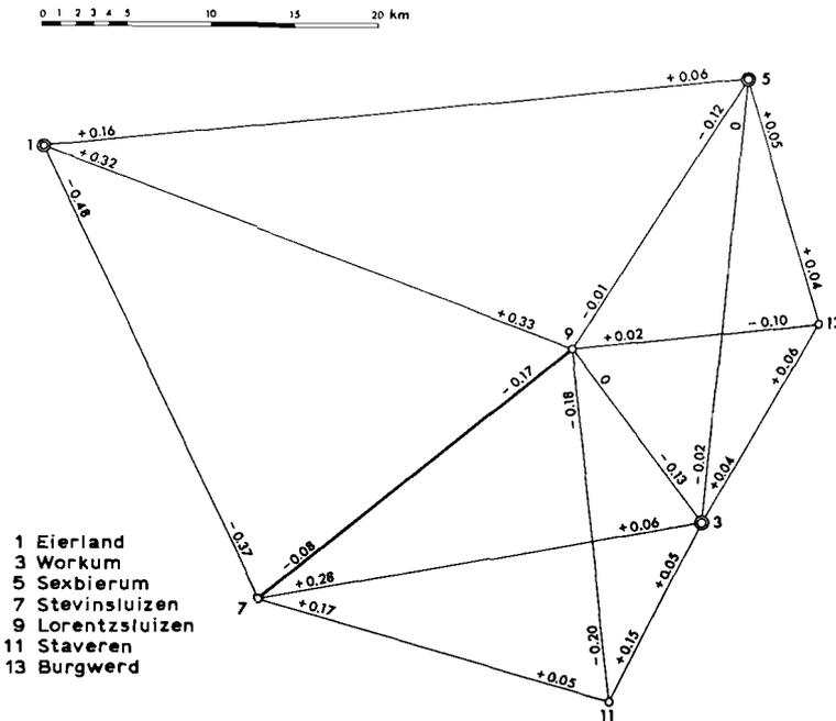
Fig. 2.1.8.  $\nabla \ln v_{9,7;1,3}$  is given as a function of  $\nabla r_{ij}$ .
