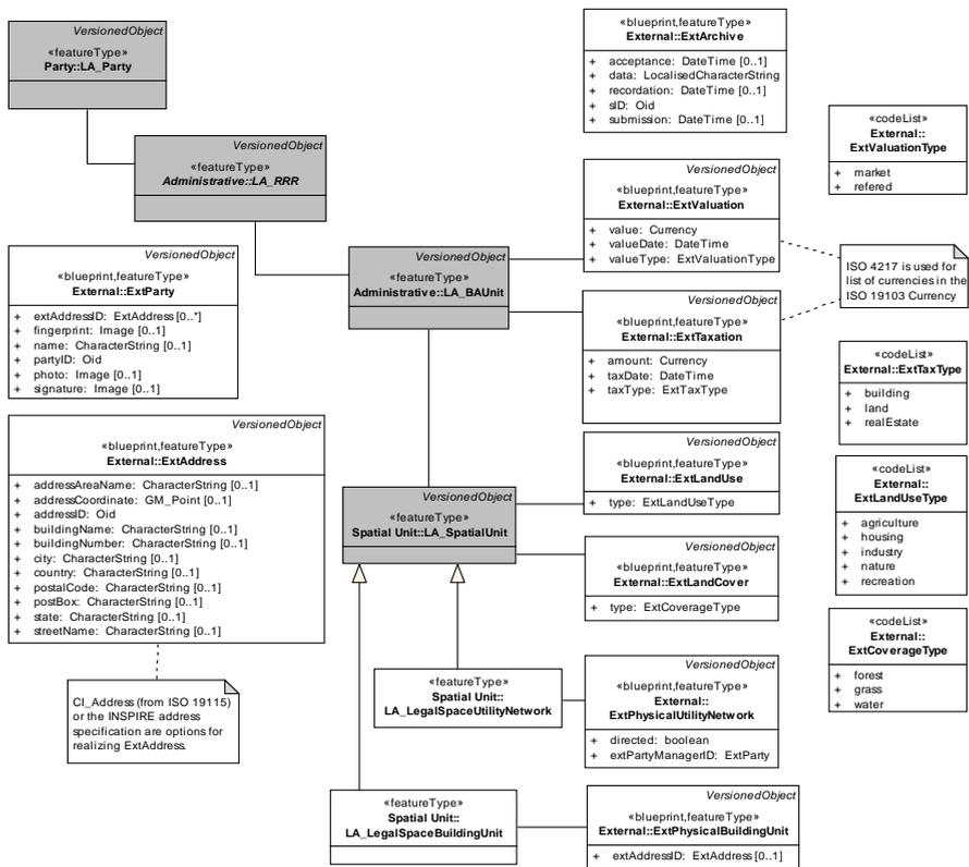
Figure 40 LADM Version C External classes ISO (2011c).
