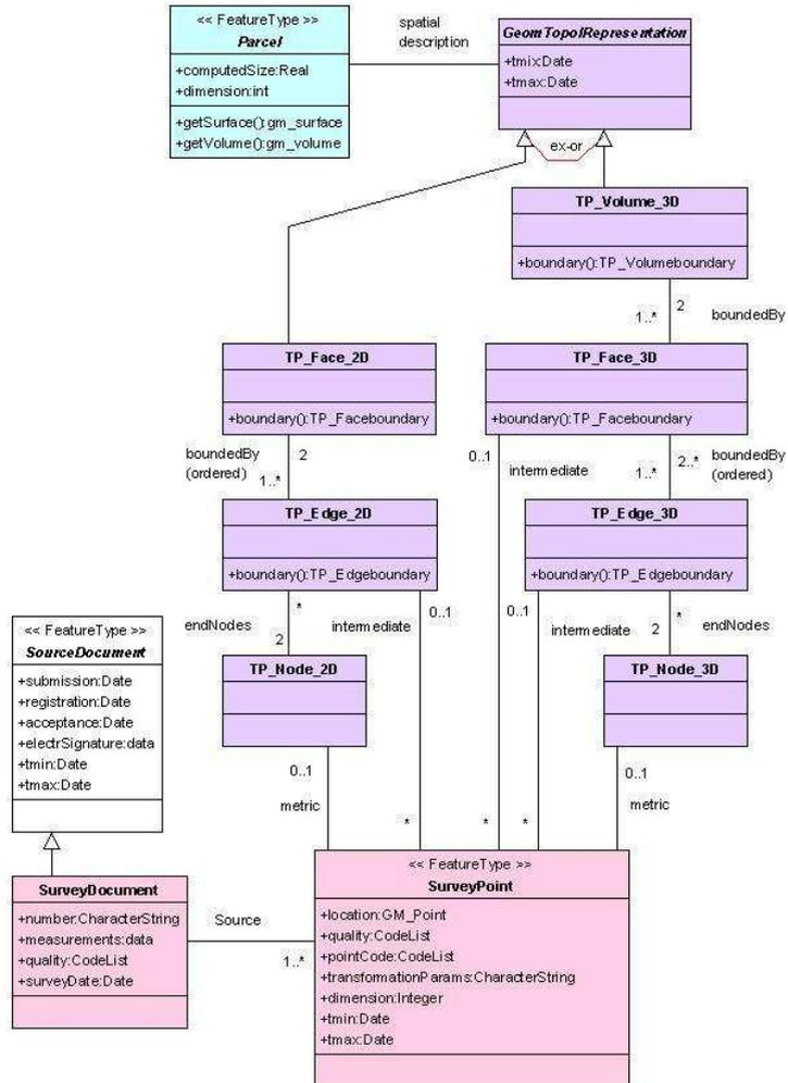
Figure 27 The Geometry, Topology and some related packages in Version B, see Lemmen, and Van Oosterom (2006a) based on Van Oosterom et al (2006b).
