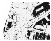
Therefore, the detected objects are removed, the shape of the line segments recomputed and new class grades determined for the remaining surface segments. The class grades are again thresholded. This process is repeated several times. The figure above shows the result after the third repetition.
