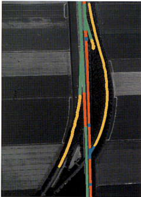
Fig. 6.6 Result of using the specialized road network model at a resolution of 0.4 m.
