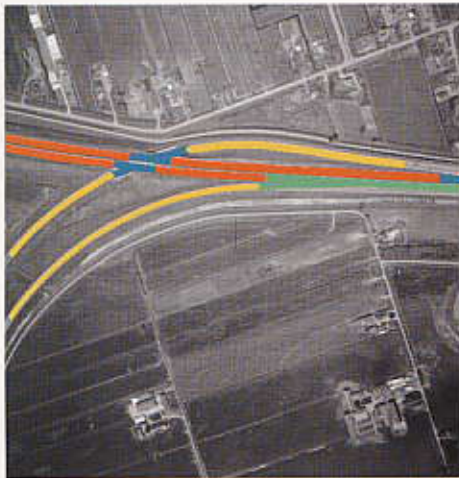
Fig. 6.1 Result of using the specialized road network model at a resolution of 1.6 m.
