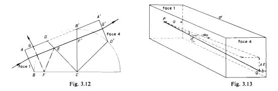
From the foregoing reasoning we can find the place at which the ray of light emerges from the pentaprism. See figure 3.13. The ray enters on face 1 at point P and emerges at point Q on face 4. We obtain from the figure:
