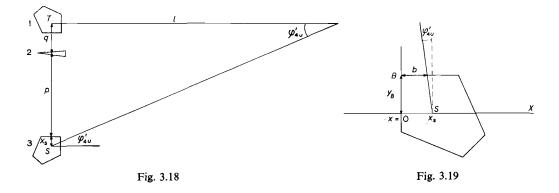
Figure 3.19 shows a horizontal cross-section through the extreme right prism (prism No. 3 in figure 3.18). We find from the figure:
