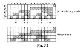
A number in the pure-binary code is represented by  $b_n b_{n-1} \dots b_2 b_1$ . A number in the Gray code is represented by  $g_n g_{n-1} \dots g_2 g_1$ .
