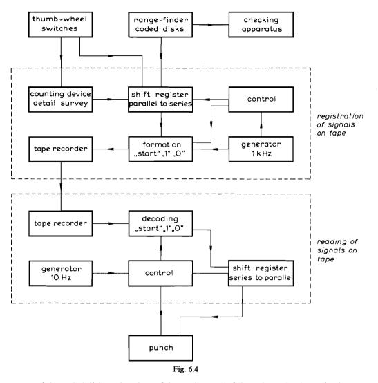
means of the coded disks, other data of the station and of the point to be determined must be registered in the memory. These data, such as station and target number, category of measurement, etc. are collected with the aid of nine thumb-wheel switches. (See section 6.3). These data are in the binary-decimal code.
