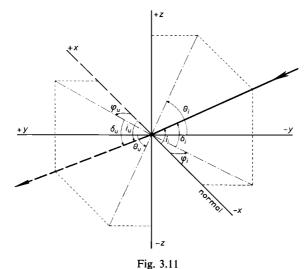
The angles  $\theta_u$ ,  $i_u$ ,  $\varphi_u$  and  $\delta_u$  of the emerging ray are expressed in the corresponding quantities of the incident ray. As the ray is refracted in the plane that passes through this ray and the normal, we find:
