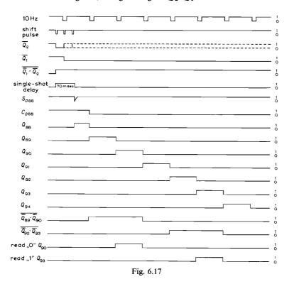
As a rule  $\overline{Q}_2 = \overline{Q}_1 = 1$ , so that  $\overline{Q}_2 \cdot \overline{Q}_1 = 0$ .
