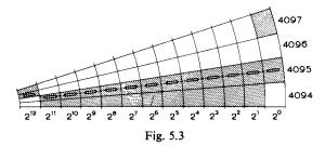
If in the inner track representing the value  $2^{12}$  the photo-electric cell is slightly ahead of or behind the correct position, an error will be made in passing from sector 4095 to sector 4096. In figure 5.3 it is not the binary number 0111111111111 = 4095 which is read, but 111111111111 = 8191, i.e. an error of 100% of the number.
