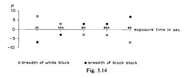
From this series the disk with an exposure time of 60 seconds was selected. This disk as viewed in its entirety was the most satisfactory in regard to halation. On grinding this glass negative to a circular shape the disk was broken. The second choice was in favour of the plate with an exposure time of 62.5 seconds. The halations were in some places slightly larger than on the disk of 60 seconds. The deviations of this disk were still within tolerable limits as will be seen in the next section.
