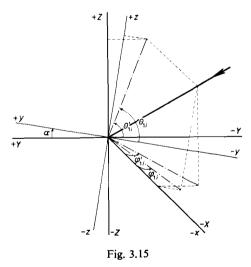
As shown by figure 3.15, the incident ray on face 1(y, z plane) of the pentaprism is given by:
