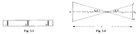
The staff is provided with three targets, whose mid points are situated 25 cm apart. If for instance targets 1 and 2 are set in coincidence in the visual field, then 25 m must be added to the distance measured.
