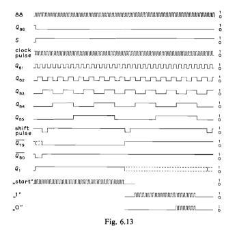
Compare the signals  $Q_{81}, Q_{82}, Q_{83}, Q_{84}$  and  $Q_{85}$  in figure 6.13. The clock pulse of ff 81 is formed by the signal  $\overline{Q}_{86} \cdot 88$ , signal 88 being the output of a generator with a frequency of 1 kHz. The shift pulse is governed by the equation:
