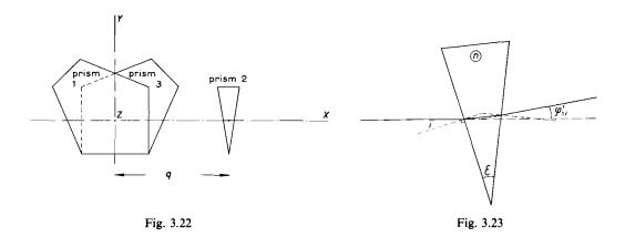
As in the case of other double-image tacheometers, the triangular prisms must be at the position of minimum deviation. The position of the prism is such that a ray of light falling parallel to the X axis acquires the minimum deviation.
