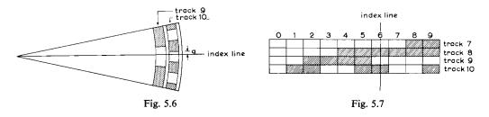
In the case of the main disk steps have been taken to ensure that in reading the micrometer the row of 10 photo-electric cells is as far distant as possible from any black-to-white transition. This mode of solution offers the greatest possible certainty that the main disk will not be erroneously read.
