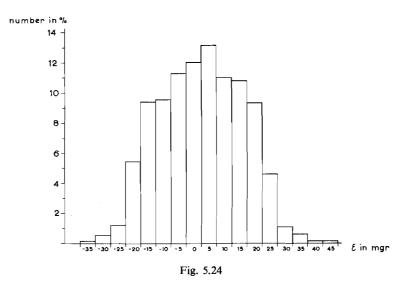
The disk for distance measurement is divided into 8192 units. Such a unit corresponds to approx. 50 milligrades. The standard deviation of the circular errors in the black-to-white
