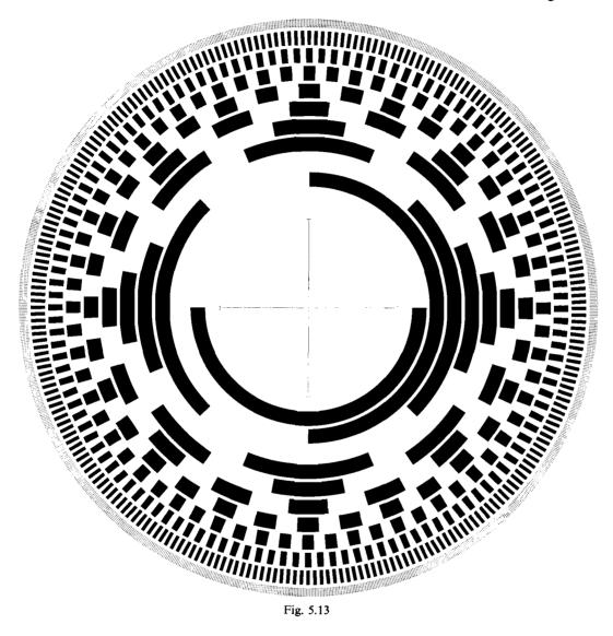
upon this material with the utmost precision by a draughtsman of the Delft Geodetic Institute. The diapositive, which was manufactured at a later stage, was a sevenfold reduction of this drawing.
