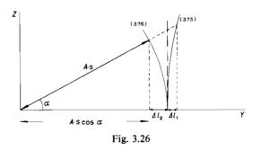
As can be seen from the figure, the curves are situated on either side of the line at which the measuring error is nil. It should be possible virtually to eliminate the error according to (3.75) by causing the rays of light to traverse a triangular prism with a very small angle of refraction, which rotates together with the pentaprisms. This can be achieved by causing face 4 of prism 1 to rotate around the Z axis (see figures 3.24).
