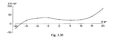
The error  $\Delta \alpha$  in the angle of inclination  $\alpha$  in figure 3.30 has a systematic trend. This renders it possible to correct a height measurement for this error in the computer. This is done with the aid of the formula  $h + \Delta h = l_{\alpha} \sin (\alpha - \Delta \alpha)$ . This gives  $\Delta h = l_0 \Delta \alpha$ .
